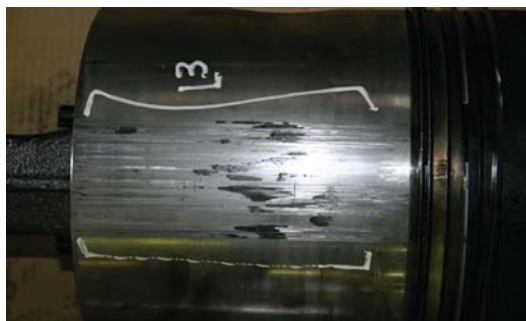
These photos of a locomotive engine indicate a severely scored liner and piston wear.
