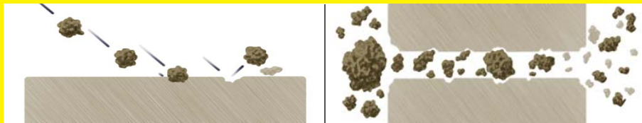
This illustration shows how particles cause damage to parts in contact. (Ref. Triple-R Oil Cleaner)
