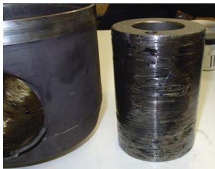
These images of a locomotive engine reveal wrist pin bearing failure.
