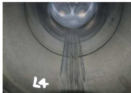
These photos of a locomotive engine indicate a severely scored liner and piston wear.
