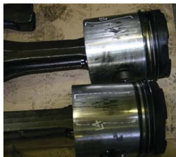
These photos of a locomotive engine indicate a severely scored liner and piston wear.
