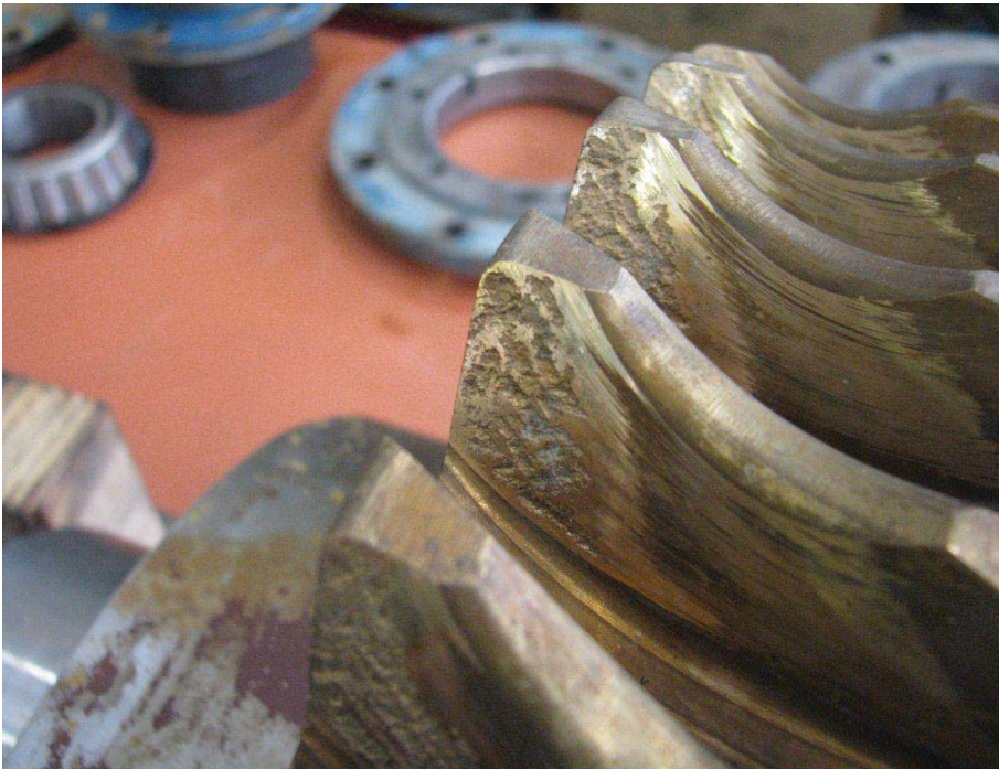
EP additives can cause damage to a worm wheel, which is usually bronze.
