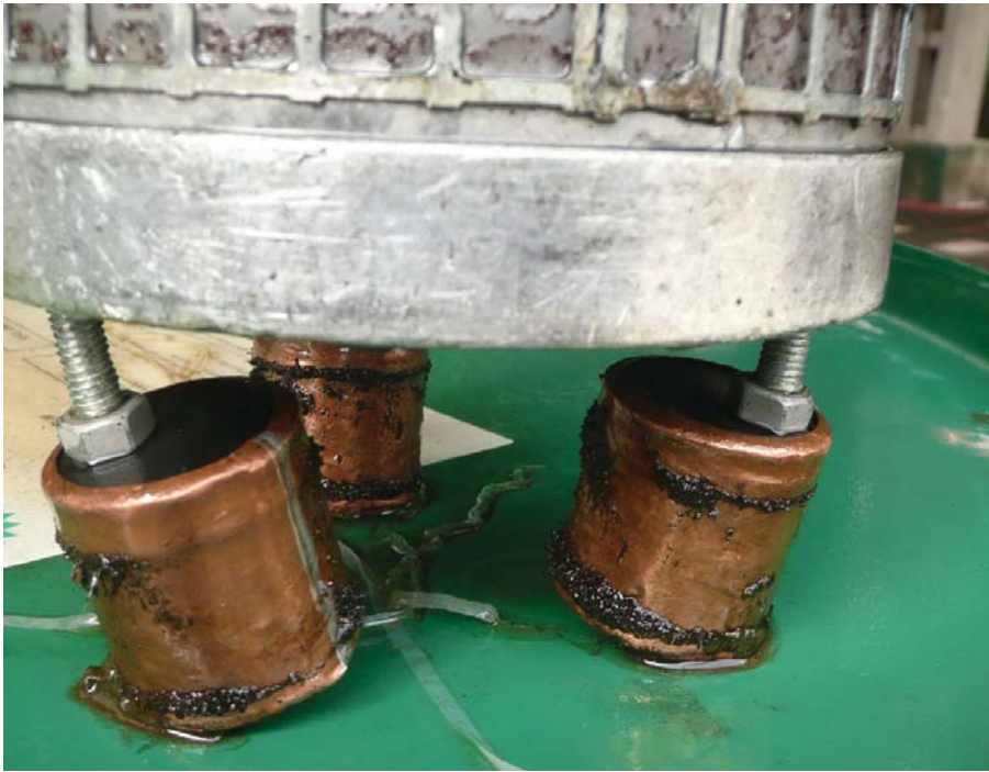
Magnetic ferrous particles attached to magnets from an oil system
