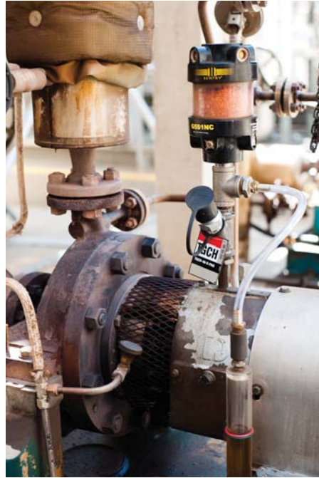
Assets are completely sealed against all contaminants and are properly labeled as to which lubricant goes into the reservoir.
