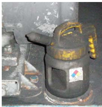
From Top: Previously, grease guns and cabinets were unorganized and dirty. Oil totes were stored outside with no protection. Top-up containers were left by the equipment and were highly contaminated.
