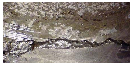
FIGURE 6. Melted Babbitt and material redeposition
