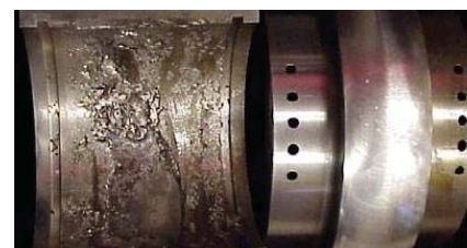
FIGURE 4. Failed pump bearing
