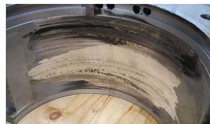
FIGURE 3. Bearing damage incurred during low-speed operation
