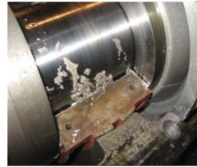
FIGURE 11. Previously melted Babbitt reformed after restoring lubrication
