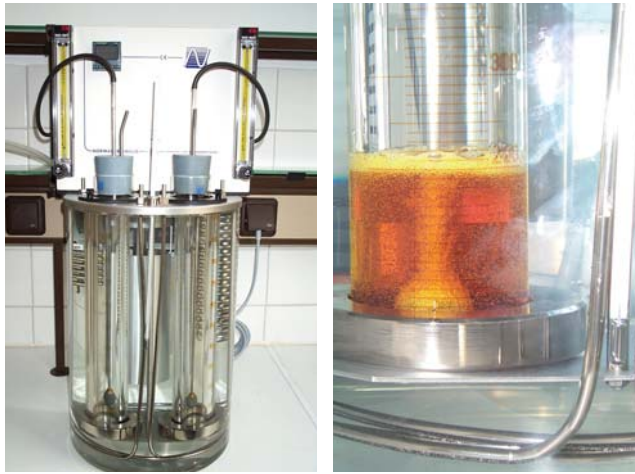
FIGURE 1. Foaming characteristics test (ASTM D892)
