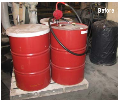
Previously, oil drums at the Georgetown mill were stored in an open building with covers or plastic bags to keep out contaminants.
