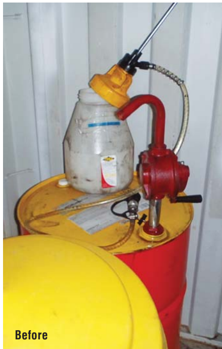
Lids often were left off reusable containers, and drum pumps were not properly sealed.
