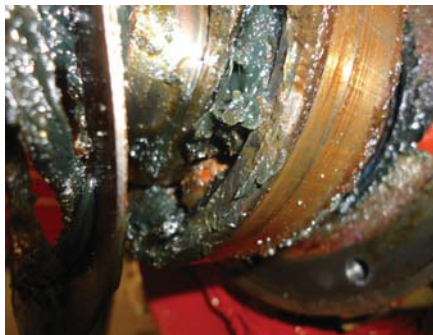
Water ingress was also an issue.
