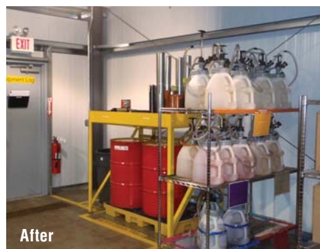
A color-coding system has been implemented in Suncoke’s new lube room including grease guns with anodized color-coded barrels and colored washers/Zerk caps.
