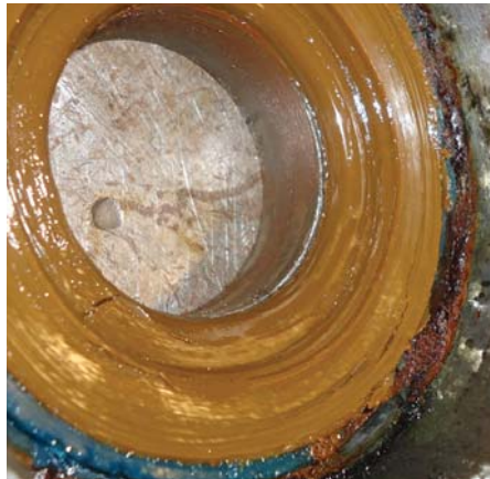
Faulty venting led to this water contamination.
