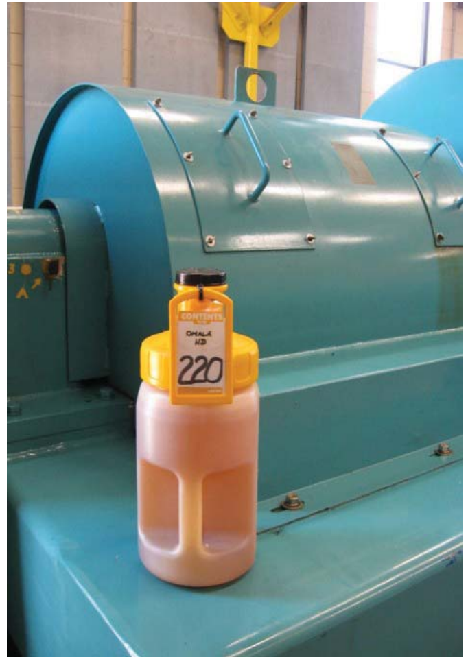
An ISO VG 220 synthetic gear oil replaced the original oil.
