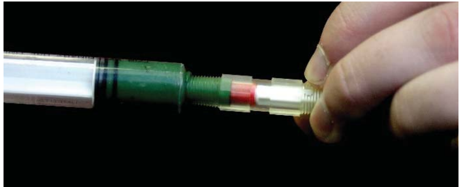
Figure 3: Filled syringe injecting grease into the Passive Grease Sampling Device easily moved while under pressure, to fill the grease sampler [Figure 3].
