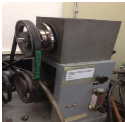
Figure 4 : Water Spray off Apparatus
