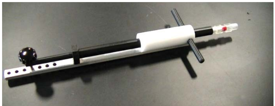
Figure 4: Grease sampler in T-handle extension
