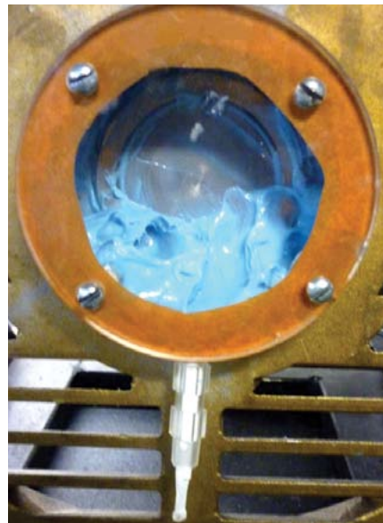
Grease mixing test stand
