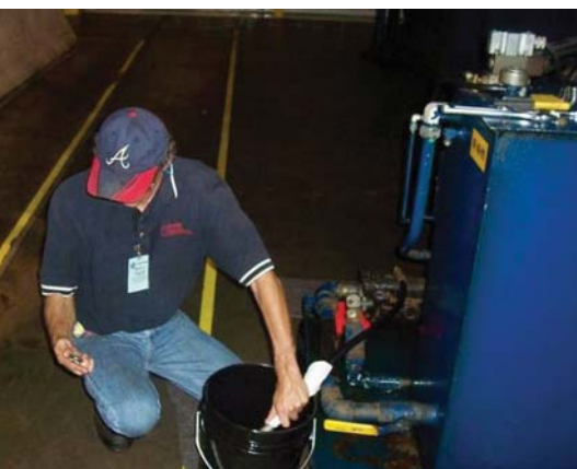
Figure 2. Check oil flow by porting the case drain line into a container of a known size and timing the flow rate.
