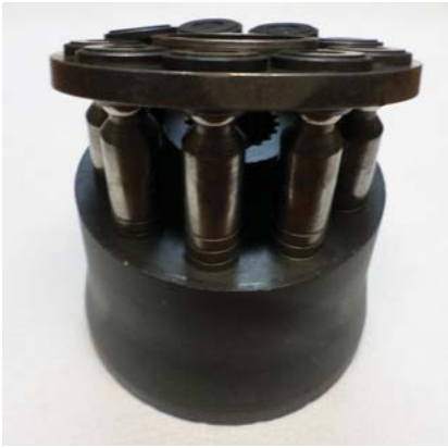
Figure 1. The tolerances between the pistons and barrel on a pressure-compensating, piston-type pump are approximately 0.0004 inch.
