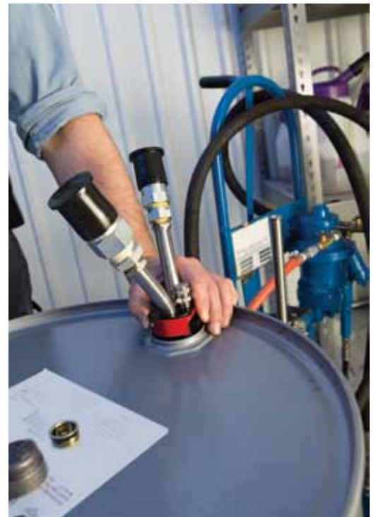
These drum-filtering adapters have a filter draw tube and return sample draw tube so the drum doesn't have to be opened to the atmosphere once the filtering process has begun.
