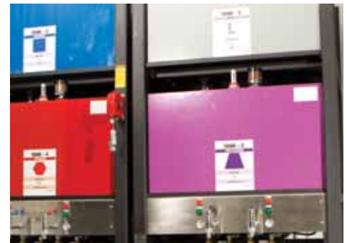
Bunge uses a color and shape-coding system to separate and identify its lubricants. These labels appear in every step of the oil-handling process.
