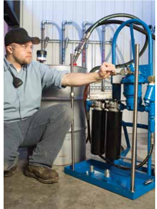
This filter cart is air-powered and has quick-connect fittings. The tube and filters have been sized so that enough ISO VG 320 oil can be used to filter the largest gearbox (180 gallons) in about five hours.
