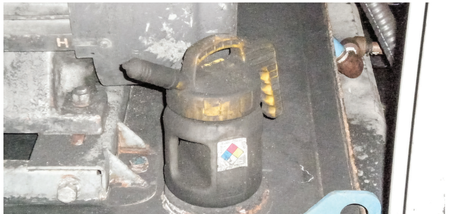
If handled correctly, a sealable and reusable container is great for topping up equipment. However, problems can occur if the container is left in the field next to equipment, not cleaned or has spouts that are not kept closed.
