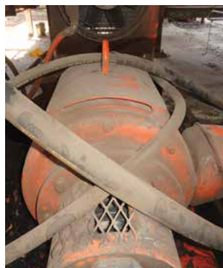
Hoses that are too long may rub on another hose or other structure.
