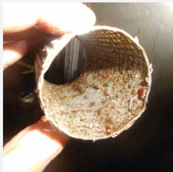
A dirty suction strainer is shown.
