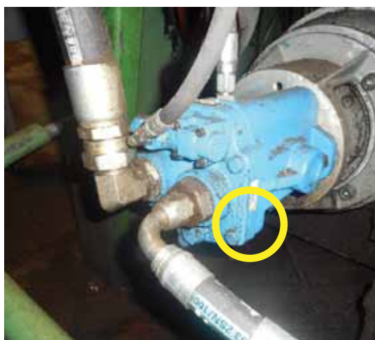
An arrow on the gear pump's housing indicates the direction of rotation.
