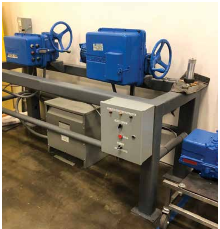
Figure 1. A motor-operated valve (MOV) lubrication test stand
