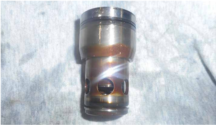
A valve that was stuck open proved to be an issue in an injection-molding machine that would not rotate at the proper speed.
