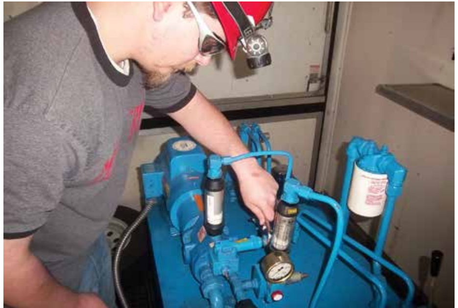
It is important to verify that all system pressures are set properly.
