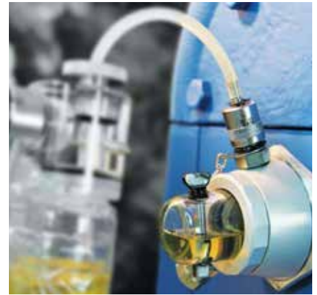
Condition monitoring pod (CMP).
