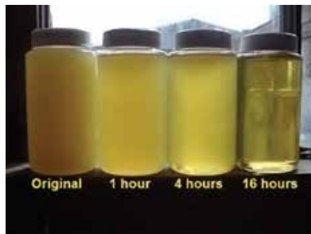
Oil purity is shown for a system before it was flushed (left) and then after one, four and 16 hours. This particular system had high water content prior to flushing.
