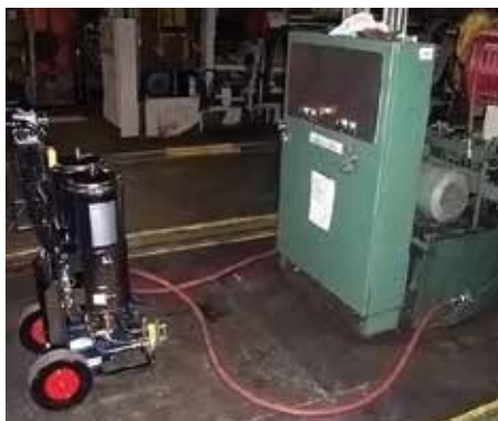
A flushing unit can be used to remove solid contaminants and water from the oil.
