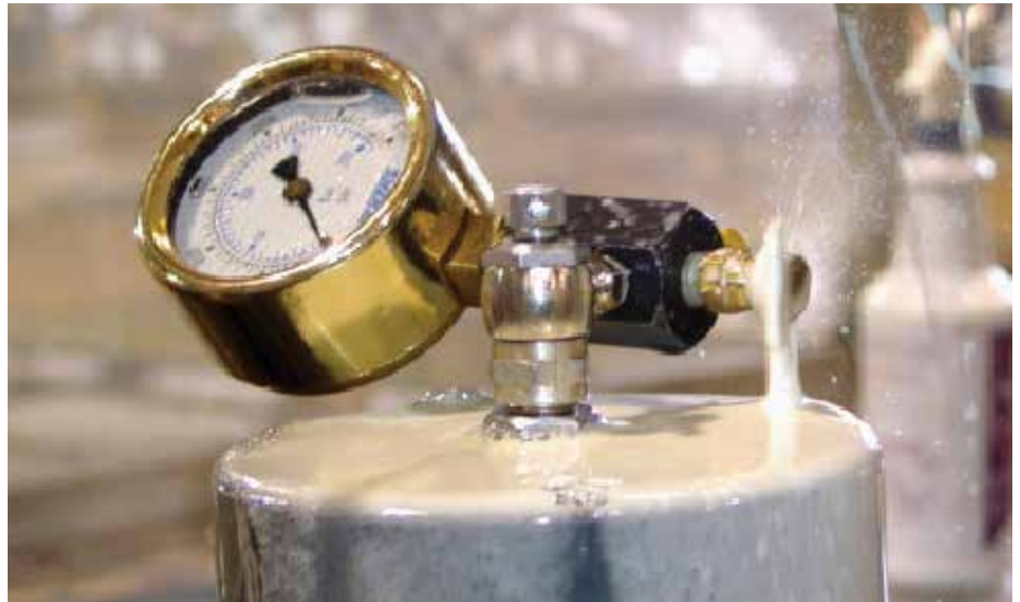
Continuous flow out of a bleed valve may indicate worn piston seals.
