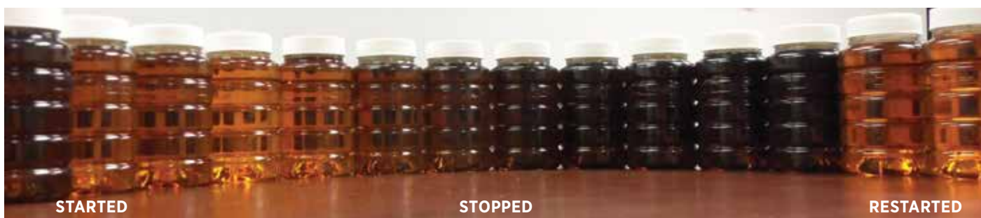
This image shows the changes in oil color when electrostatic filtration was started, stopped and restarted.
