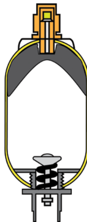
If a bladder accumulator loses its charge, the bladder may be pushed to the top of the shell and become ruptured by the Schrader valve assembly.
