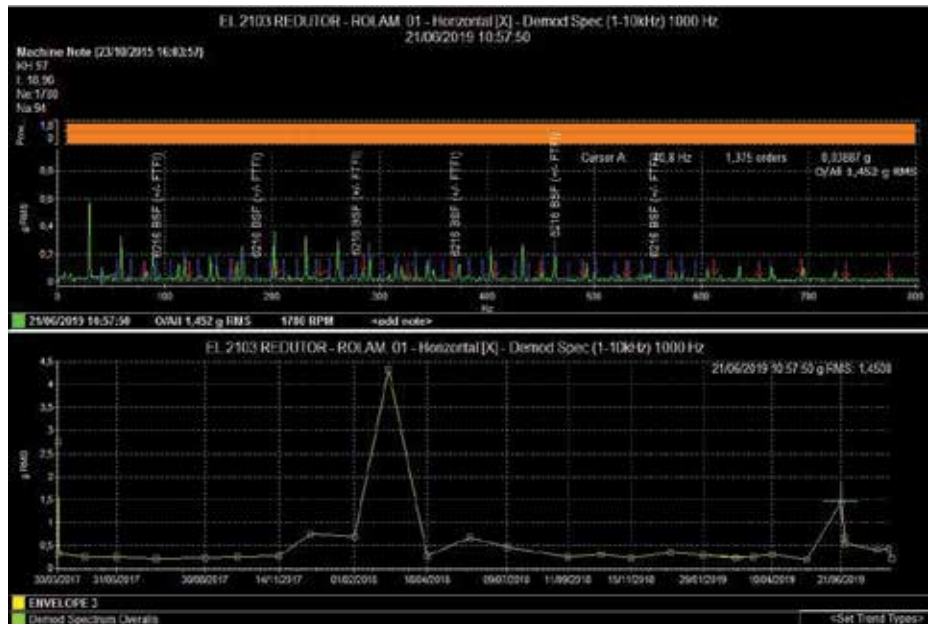
Figure 12. The vibration spectrum for the lift gearbox
