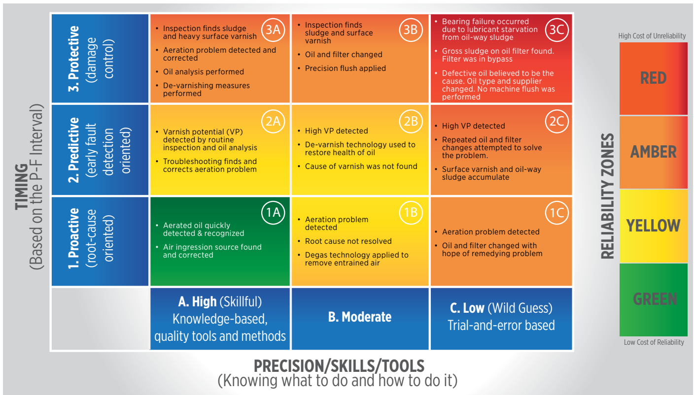
Figure 3. A detection zone table used to illustrate how condition monitoring can detect and respond to failure in different ways
