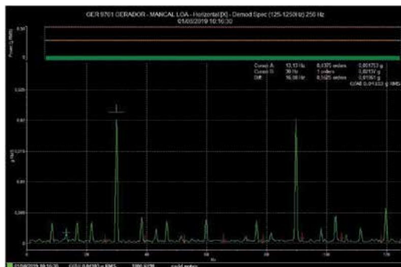
Figure 3. Oil instability frequency
