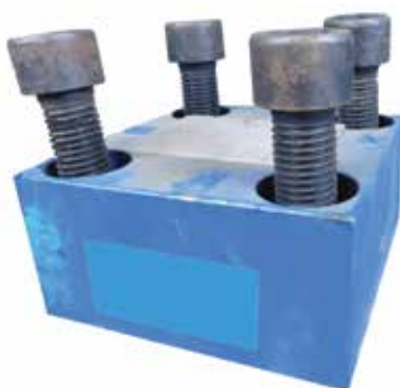
Figure 6. Most logic valves are mounted beneath a cover that's secured by four bolts.
