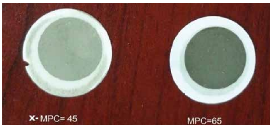
FIG 2. Sample of oil patch for a gas turbine in petrochemical plant.
