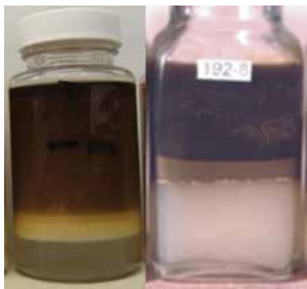
Figure 3. Two different samples exhibiting all four states of water and oil. Note the milky white appearance of the free water phase in both samples. Many oil impurities transfer to free water including some dead additives. Seeing what's in the water phase can provide supplemental information about other contaminants and the condition of the oil. Pay attention! The band in the middle of both samples is the oil-in-water emulsion. How thick is this band? Does it diffuse or does it have good definition?
