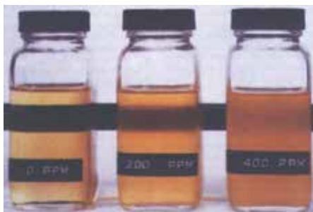
Figure 1 Shown here is dry hydraulic fluid on the left and increasing amounts of emulsified water (water-in-oil) to the right.
