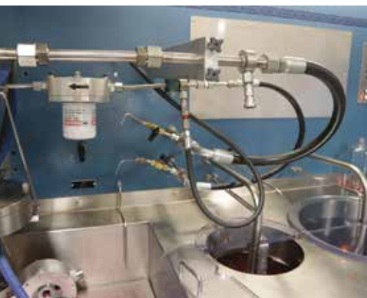
Figure 4. The left-side test sink shows a small spin-on filter mounted and ready for testing.
