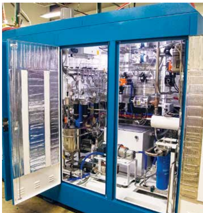
Figure 1. Interior multipass system circuits and components. The dilution system and particle counters are mounted on the left interior panel.
