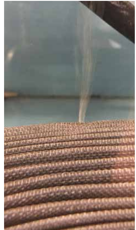
Figure 7. The test bench on the left is used for bubble point testing (ISO 2942). The image to the right shows a stream of bubbles from a defective opening in the filter media. The air pressure reading when the first bubble appears is recorded as the bubble point.
