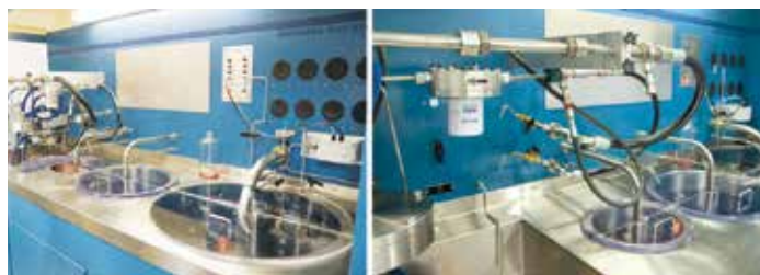
Figure 2. Above the sink on the left is where the filter being tested is mounted. The circular middle sinks are filter test system reservoirs. The larger injection system reservoir is on the far right.
