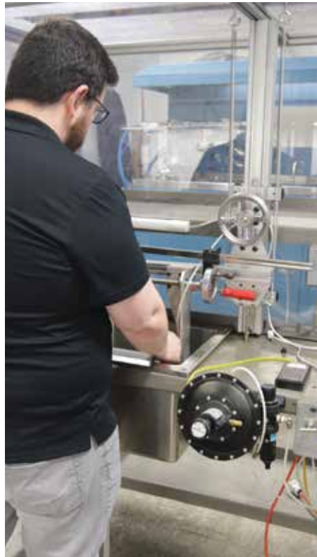
Figure 7. The test bench on the left is used for bubble point testing (ISO 2942). The image to the right shows a stream of bubbles from a defective opening in the filter media. The air pressure reading when the first bubble appears is recorded as the bubble point.
