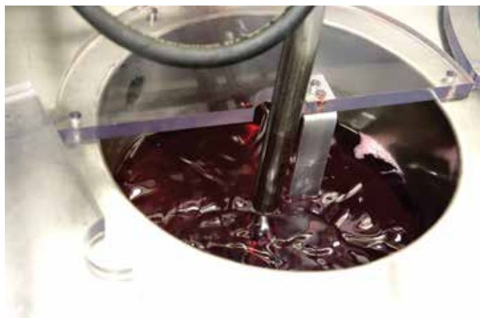
Figure 3. Funnel-shaped sinks achieve turbulent flow, enabling controlled homogenous distribution of particles across a range of sizes during the test sequence.
