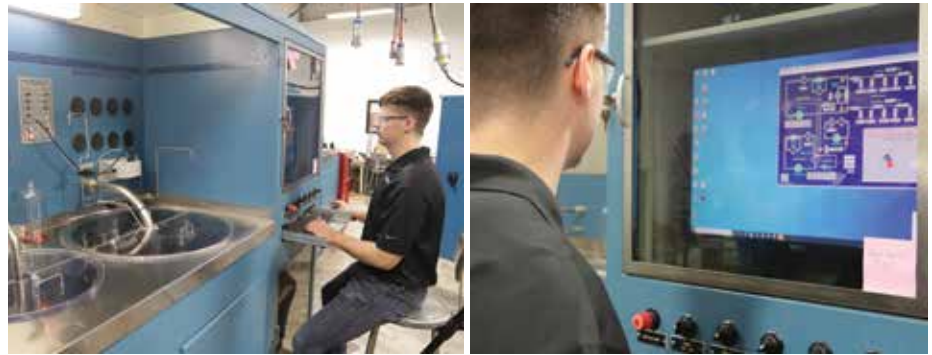
Figure 5. Filter tests conditions are defined at the computer station before the start of the test. This is followed by a warm-up stage. During the test, data appears on the screen circuit diagram.
