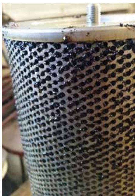
Figure 1: This filter is loaded with sludge from a system with severe electrostatic discharge issues.
