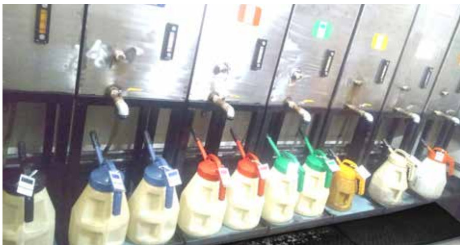
Figure 3. Dedicated colour-coded oil dispensing containers
