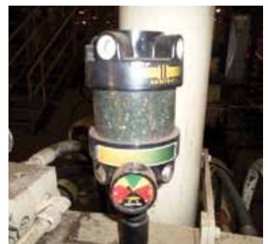
A desiccant breather can be used to remove moisture from the air before it enters the tank.
