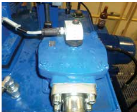
Filters often are connected in the return lines of a system's directional valves.
