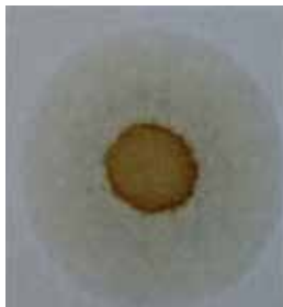
This blotter shows rust from a lubricant contaminated with water. Oil analysis found 397 parts per million (ppm) iron. Water is not generally observable on non-engine blotters. The base oil properties looked normal.
