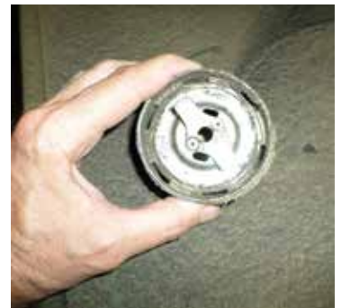
Some hydraulic units have an inexpensive breather that doubles as a fill cap.
