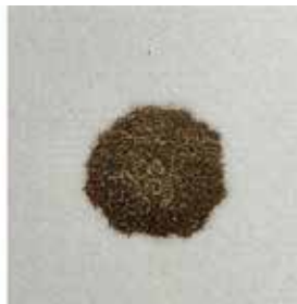
This is an ISO VG 220 gear oil. The 870 ppm iron was mostly silt-sized wear debris and rust. The lubricant was probably heavily filtered. The base oil and other properties appeared normal.
