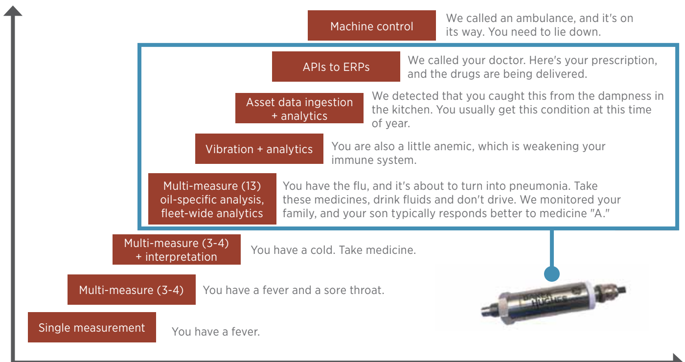
This illustration offers a glimpse into the future of the lubricant monitoring industry along with a corresponding health analogy.
