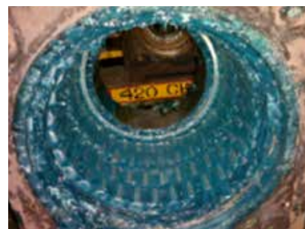
Used new grease in Roll Chock
