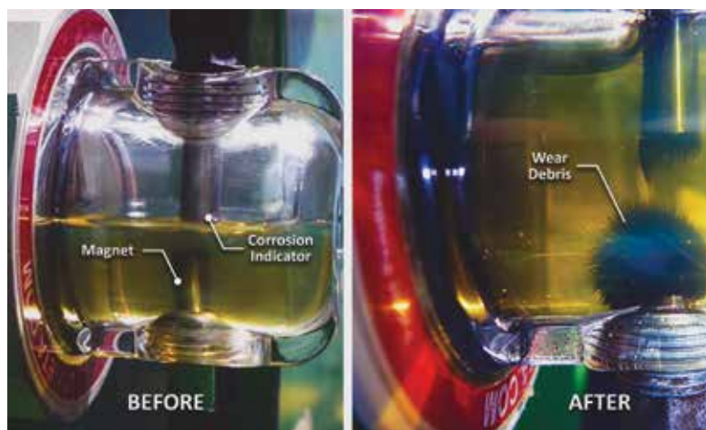
Figure 3 – After only 58 hours, large amount of ferrous wear debris can be seen on the CMP’s visible magnet. Notice that the steel corrosion indicator has also become magnetized and has also collected debris.
