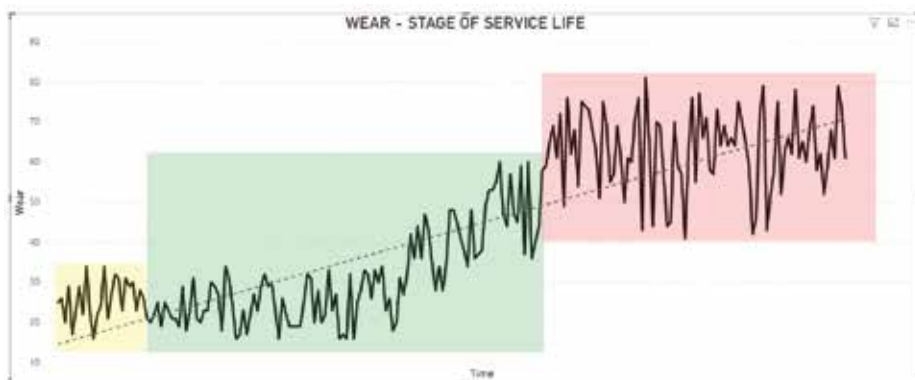
Figure 2: Iron (Fe) wear values from a set of samples of 63 gearboxes
