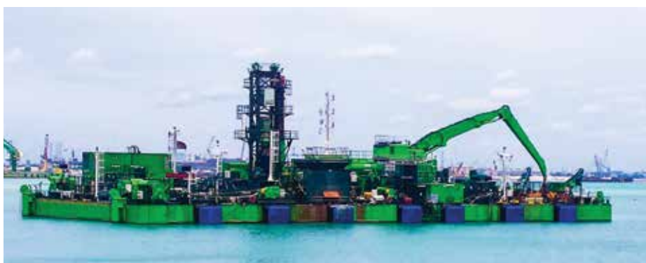
Figure 1 - The first and only all-in-one rock mound construction vessel
