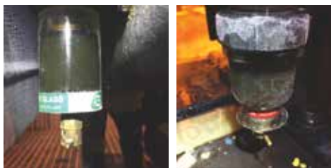
Figure 3. The bowl on the left shows sediment buildup and the bowl on the right shows water buildup. Bottom Sediment & Water bowls are a key tool for recognizing a problem exists and excluding the problem on the spot.
