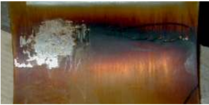
Figure 4: Deposits and severe metal wear occurring in the hottest zone of the bearing surface.
