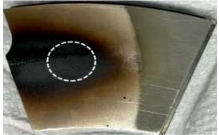
Figure 2: Bearing pad showing a dark patch of deposits at the highest load zone of the bearing. Deposit characterization of this deposit revealed that it was composed of phosphorus-based EP deposits.
