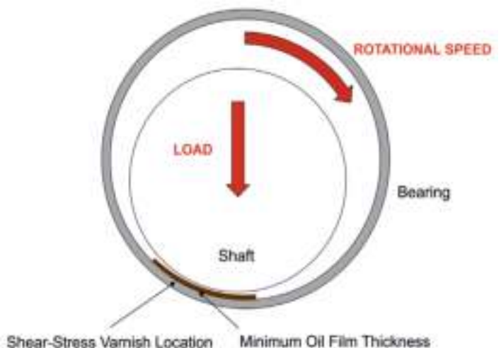
Figure 8: Illustration showing the varnish forms at the minimum oil film thickness point and the two primary forces influencing shear-stress are load and rotational speed.
