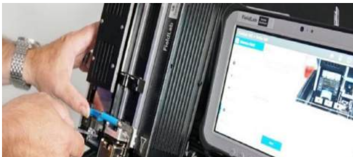
Figure 3 outlines the two-step process for extracting >4 micron particulate from in-service oil samples and measure the elemental com-
