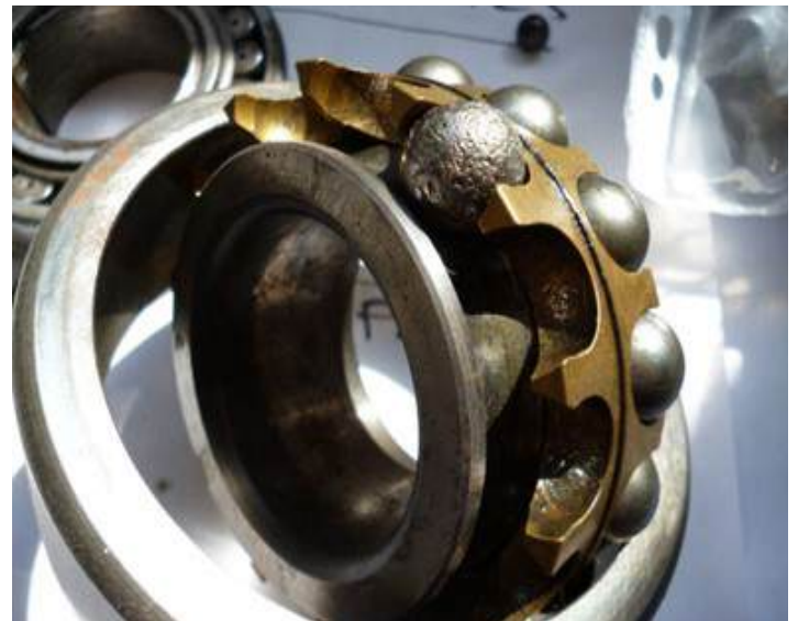
Figure 04 Revealed bearing damage from a teardown inspection
