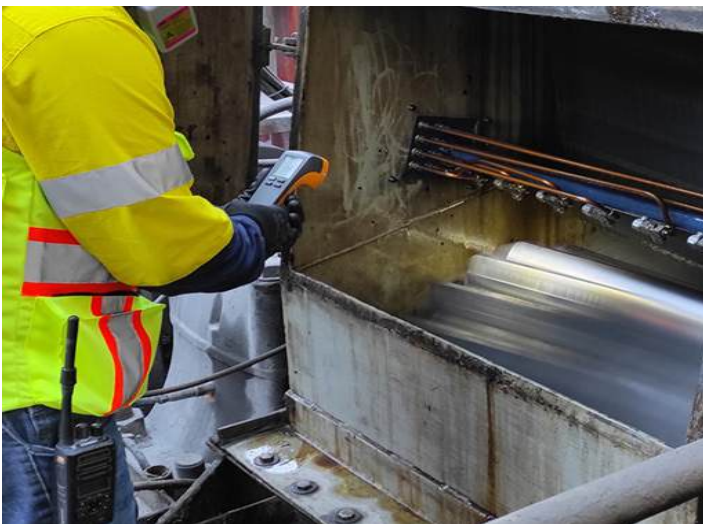
Figure 03 Stroboscope gearbox inspection
